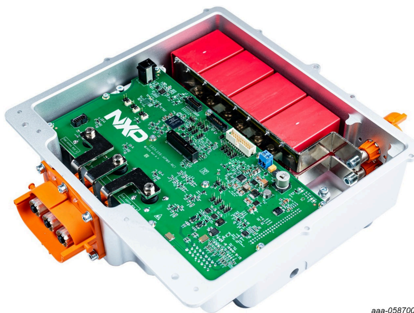
Figure 1. ECU made in collaboration with Vepco based on EV-INVERTGEN3 boards
