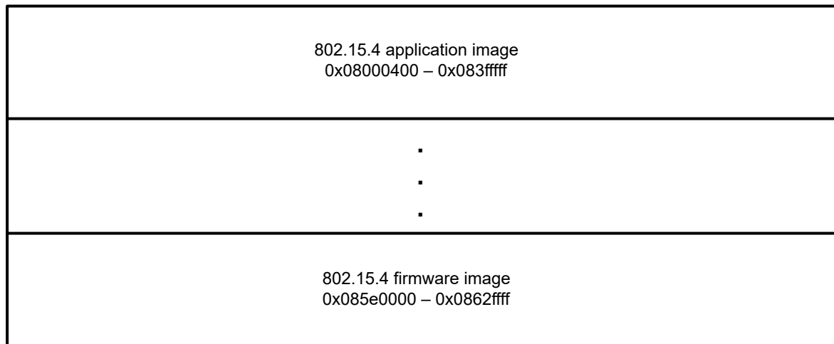
Figure 5. Partitions of FlexSPI NOR flash
