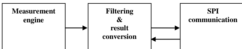
Figure 2. Block diagram of the data acquisition firmware
