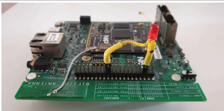
Figure 9. LED connected to GPIO5_IO13
