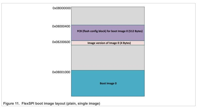
The FlexSPI boot image address must be at  $0 \times 0800\_1000$  (XIP, loading, and executing address are the same). Write a valid FCB block in  $0 \times 0800\_0400$ . The boot ROM fetches FCB via 1-bit SPI mode, configures the NOR FLASH with FCB information, and tries to boot NOR FLASH image.
