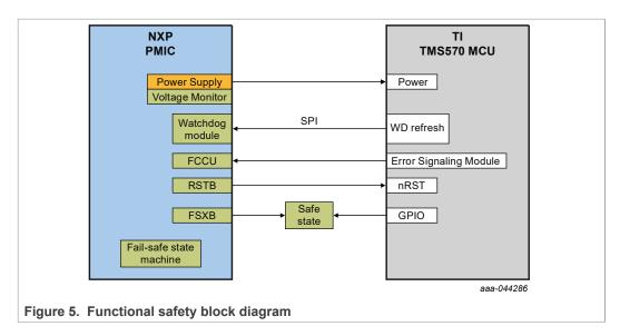
FS26, FS45 / FS65 and FS85 integrate Challenge WD, allowing monitoring of the TMS570 through the serial-parallel interface (SPI).
