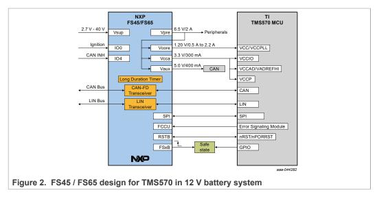
Vcca and Vaux can output 3.3 V or 5 V, depending on the resistor value on the SELECT pin. The Vcca output current capability is 300 mA, with 3% accuracy, with external PNP, and 100 mA, with 1% accuracy, with internal PNP (leave VCCA B open and tie VCCA E
