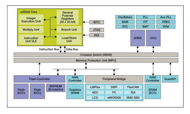
View additional information for Ultra-Reliable MPC560xS MCU for Automotive and Industrial Instrument Clusters.
