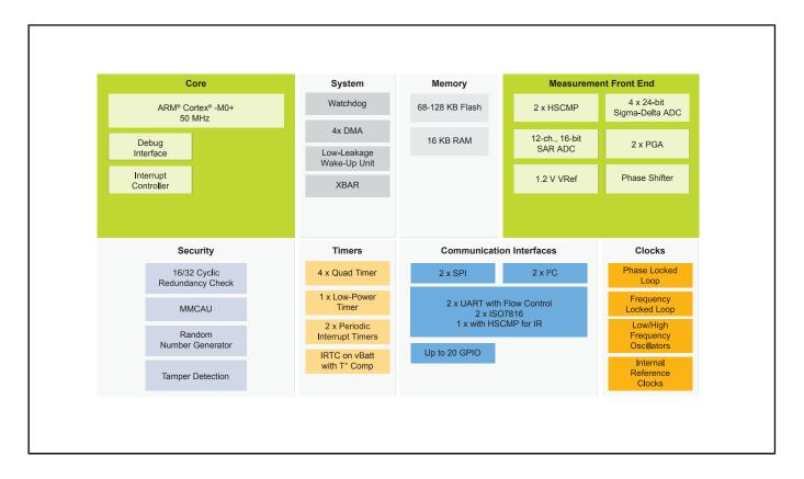
View additional information for 50 MHz, Mainstream Precision Metrology Microcontrollers based on Arm® Cortex®-M0+.
